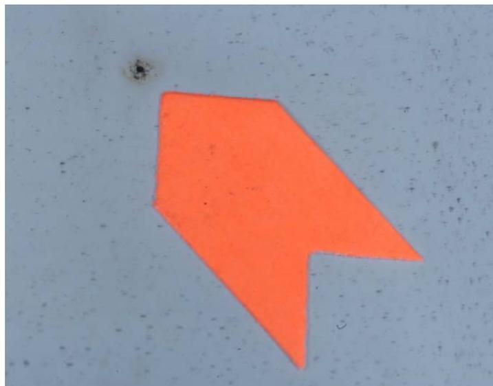
*Figure 9: A Micro-shorting Location on a Separator, the size is approximately 1mm. (Mikolajczak et al., 2011)*
