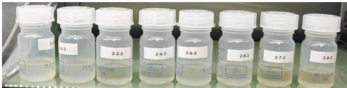
*Figure 11. The Electrolyte Samples Taken on Day 3. The Dark Colour Indicates the Samples with High Impurities*
